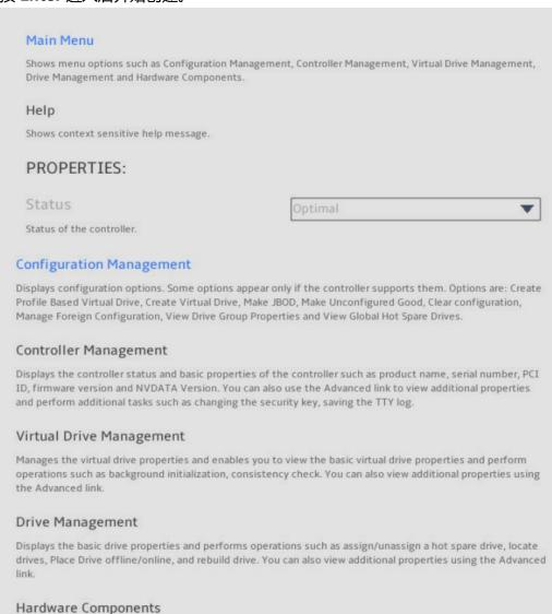
Displays the battery and enclosure status if applicable. You can also view additional properties and perform additional operations using the Advanced link. Some options will appear only if the controller supports them.
