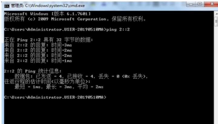
IPV6子网2的SW1也可PING通IPV6子网1的PC:
