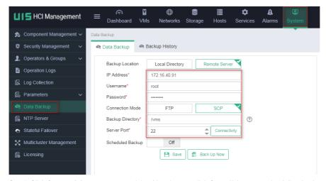
Step2:Click Connectivity to test connectivity. After the test, click Save. If the connection fails, check whether the IP address, password and backup path are existent.
