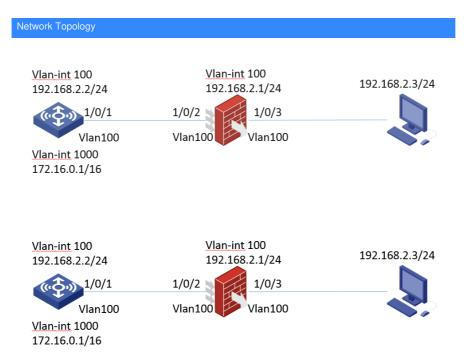
The network topology is shown in the figure above. The int-vlan 1000 of wireless controller is used as the gateway of  $\,$  wireless clients. The 1 / 0 / 2 and 1 / 0 / 3 of firewall are all in the trust domain. The int-vlan100 is the three-layer interface of firewall, which is the gateway of terminal PC. The int-vlan10 0 also belongs to the trust domain. The 1/0/2 and 1/0/3 of firewall are two-layer interfaces, which permit vlan100 to go through.
