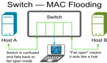
Figure 6, Switch-MAC Flooding
