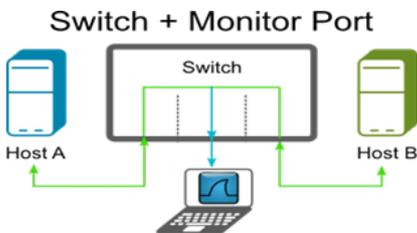
Figure 7, Switch+ Monitor Port
