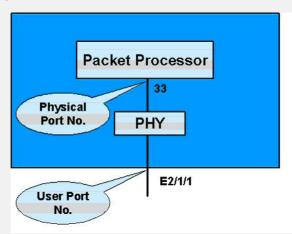
Upon link aggregation, choice of the active port is based on the subscriber port. If yo u use the command link-aggregation Ethernet 4/1/1 to Ethernet 4/1/5 both to cond uct port aggregation, the active port is Ethernet 4/1/1 whose port No. is the smallest. While sending packets outbound, select the port with the smallest physical port numb er. As the physical ports and the logical ports are not numbered in the same order, th e port to send the packets may not be the primary port.
