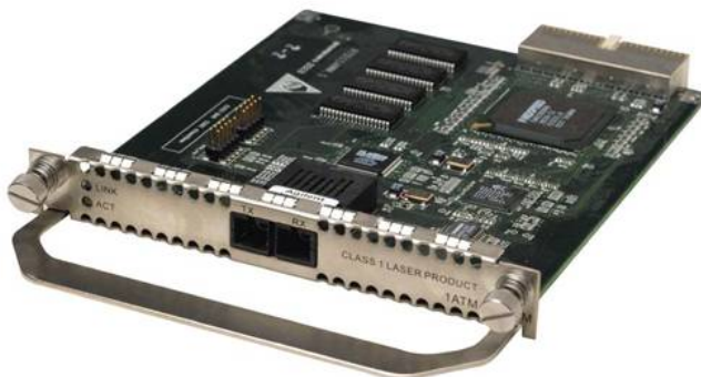
SC type fiber connector appearance
