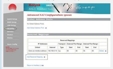
**Step5** Add another mapping filled with camera address, Transport type and the port 4321
